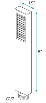
Flow Rate: 2.0 GPM / 7.6 LPM
